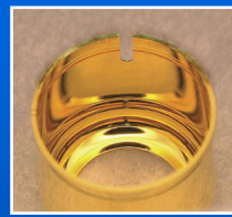
Au and depleted U hohlraums with milled features
