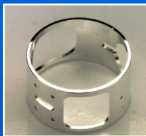
Al components with milled diagnostic features
