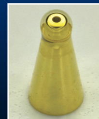
Shock timing cone and shell target
