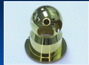
Spherical hohlraum with diagnostic ports
