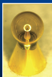
Fast Ignition cone and shell target
